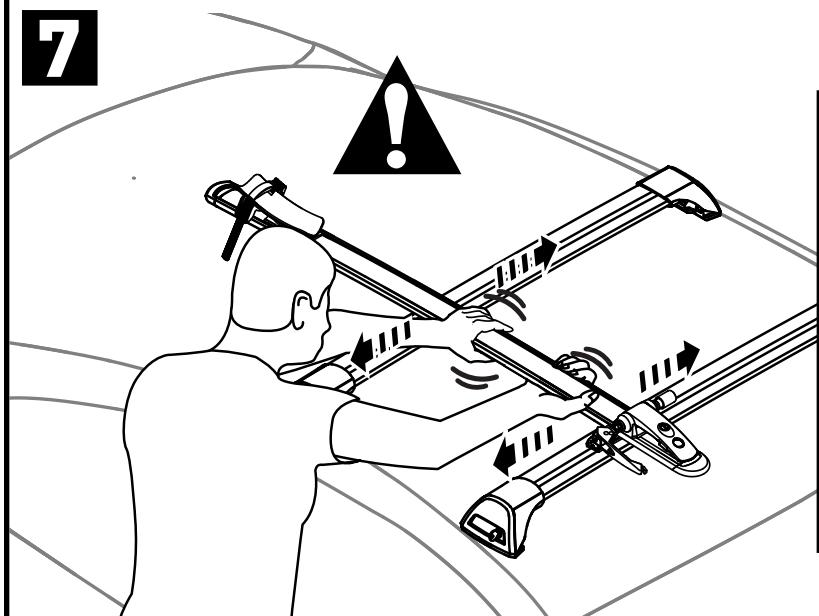
Test the installation. If the carrier moves remove the carrier (see steps 19 through 21) Then repeat steps 2 - 6.
