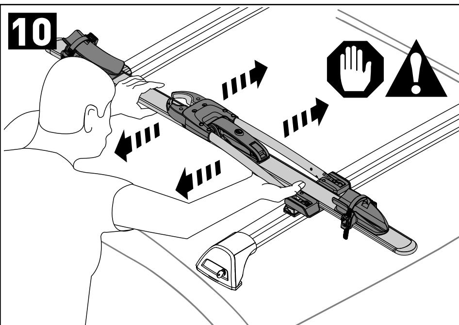
Test the installation. If the carrier moves remove the carrier (see steps 24 through 26) Then repeat steps 2 - 9.
